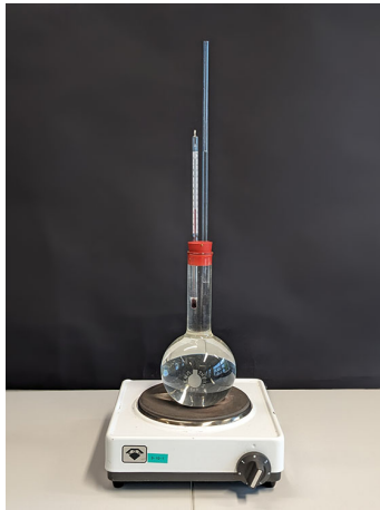
(a) Measuring the height of the column of water for different temperatures.
